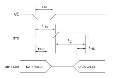
Figure 4 - High Pulse for R/C - Outputs Enabled While R/C is High, Otherwise High Impedance
