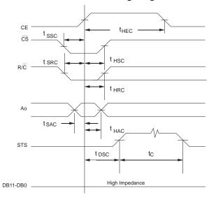
Figure 2 - Read Mode Timing Diagram
